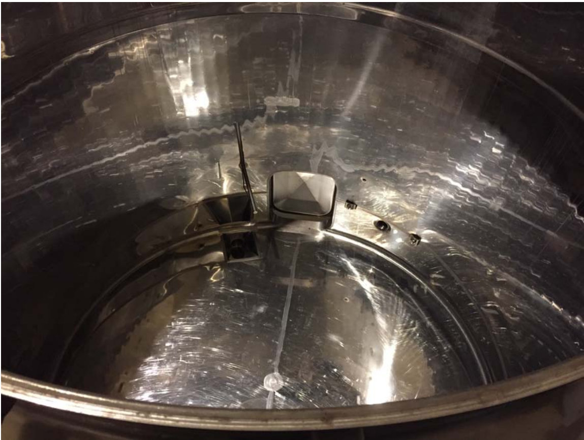
~ This is the view down into one of the fermenters from above the catwalk. Although it doesn't look that deep, it's probably about 10-12 feet deep. Visible is the door which they use to assist in cleaning the tank ~
